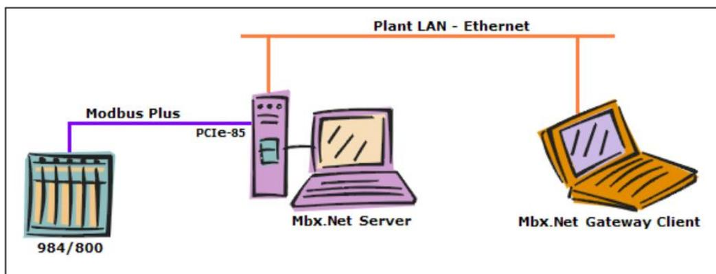
In this setup, the tower system uses the MBX Driver and a PCIe-85 card to communicate over Modbus Plus to the 984 controller. The tower is also running the Mbx.Net Server, making it the server system.
