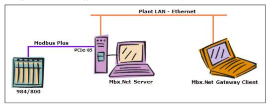
The figure below shows a typical use of the Mbx.Net Gateway Driver.
