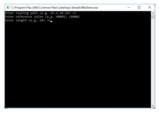
Enter the *routing path* of the node you want to read from. This may be an IP address, a Modbus routing path or node number, depending on the type of network. For more details, refer to the MBX Demo documentation for the device type you are connecting to on the server.
