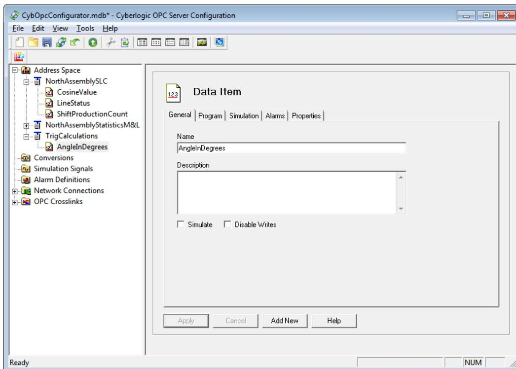
In the figure above, you can see that we've added the data item CosineValue to the NorthAssemblySLC device. This gets its data from the SLC, and holds the cosine value that we want to convert to an angle.
