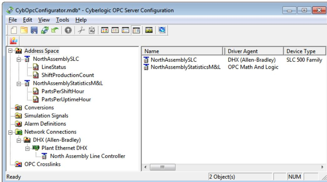
In the OPC server shown above, NorthAssemblySLC is an ordinary device associated with a SLC-500 controller. It contains data items LineStatus and ShiftProductionCount.
