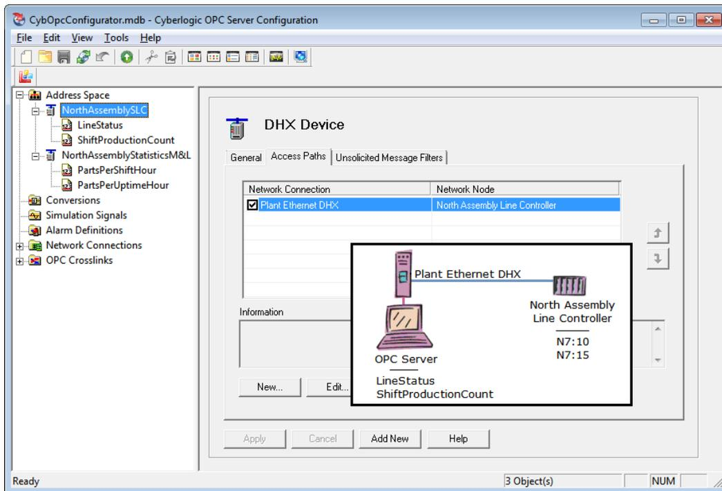
When you configure a conventional data item, you place it in a device with an access path to a PLC, as shown in the figure above. The value of the data item simply reflects the value of a register you specify in that controller.
