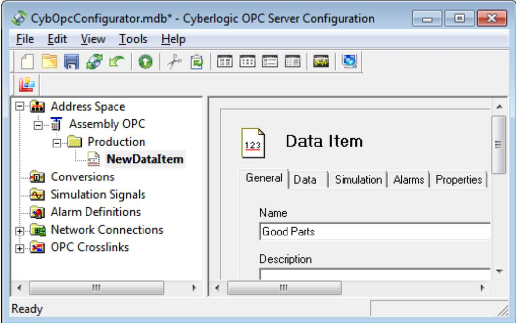
The folders and data items look just like those in a device associated with a PLC. But instead of bits or registers within a PLC, these data items link to data items in the OPC server you are connected to.
