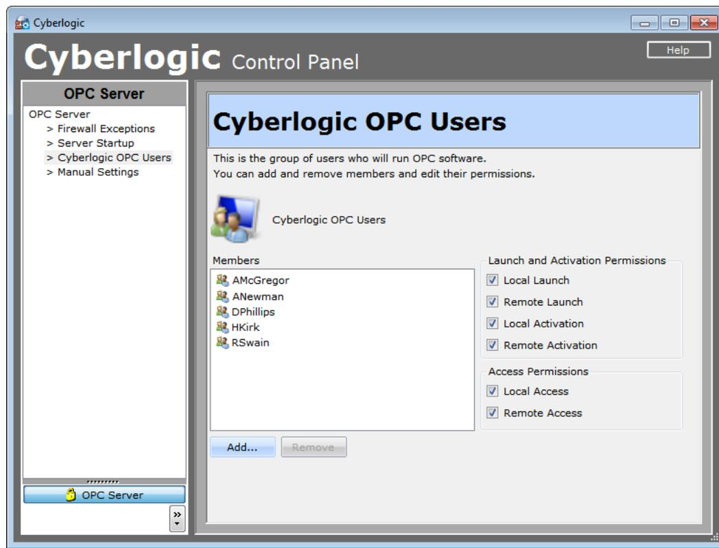
During the product installation, a users group called Cyberlogic OPC Users is automatically created and added to the security settings for the Cyberlogic OPC Server. By default, only the user that installed the software is added to this group, however, other users can also be added later. Using a group makes it easy and efficient to apply the needed permissions to every user who will need to run the Cyberlogic OPC server software.
