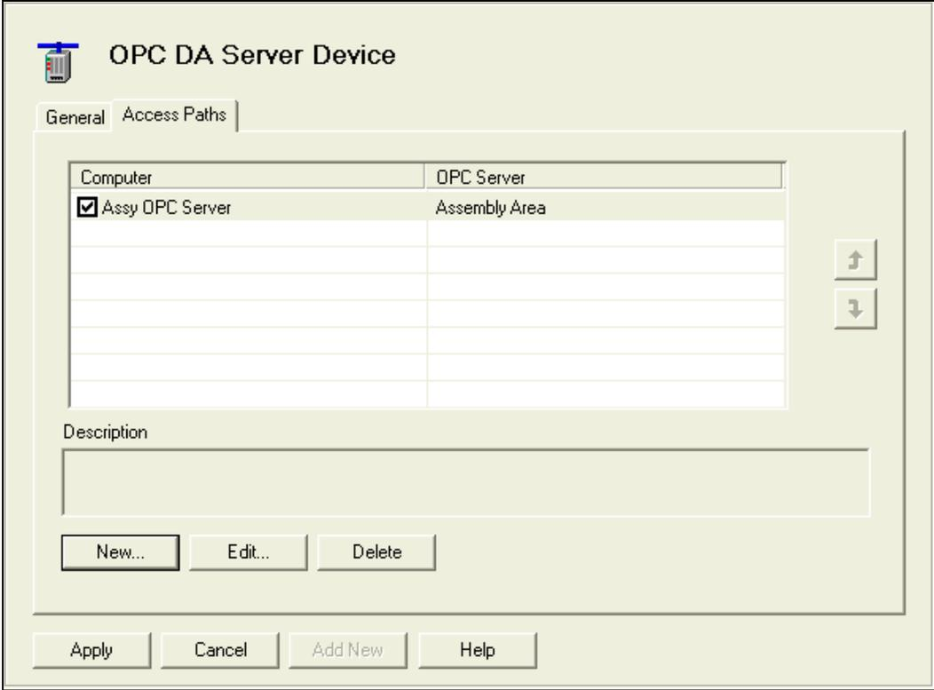
The OPC DA Server Device has access paths, just like any other device. And just like any other device, you can configure two or more access paths for redundancy.
